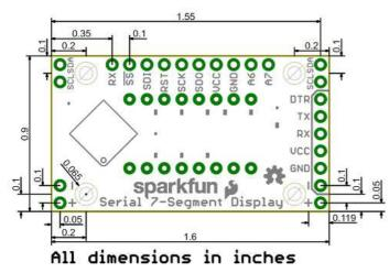
All through-hole pins on the display are spaced by a breadboard standard 0.1 inches.
